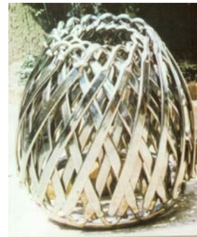
Fig. 5 – The first 50 kW air-cooled solar receiver designed by Giovanni Francia, installed for testing at the Sant'Ilario station in August 1979 (Francia Archive)
